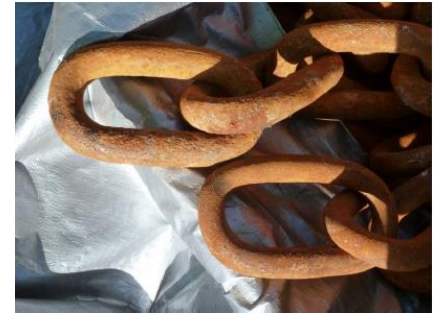
Corroded chain from USCG ATON Buoy (MMC)
